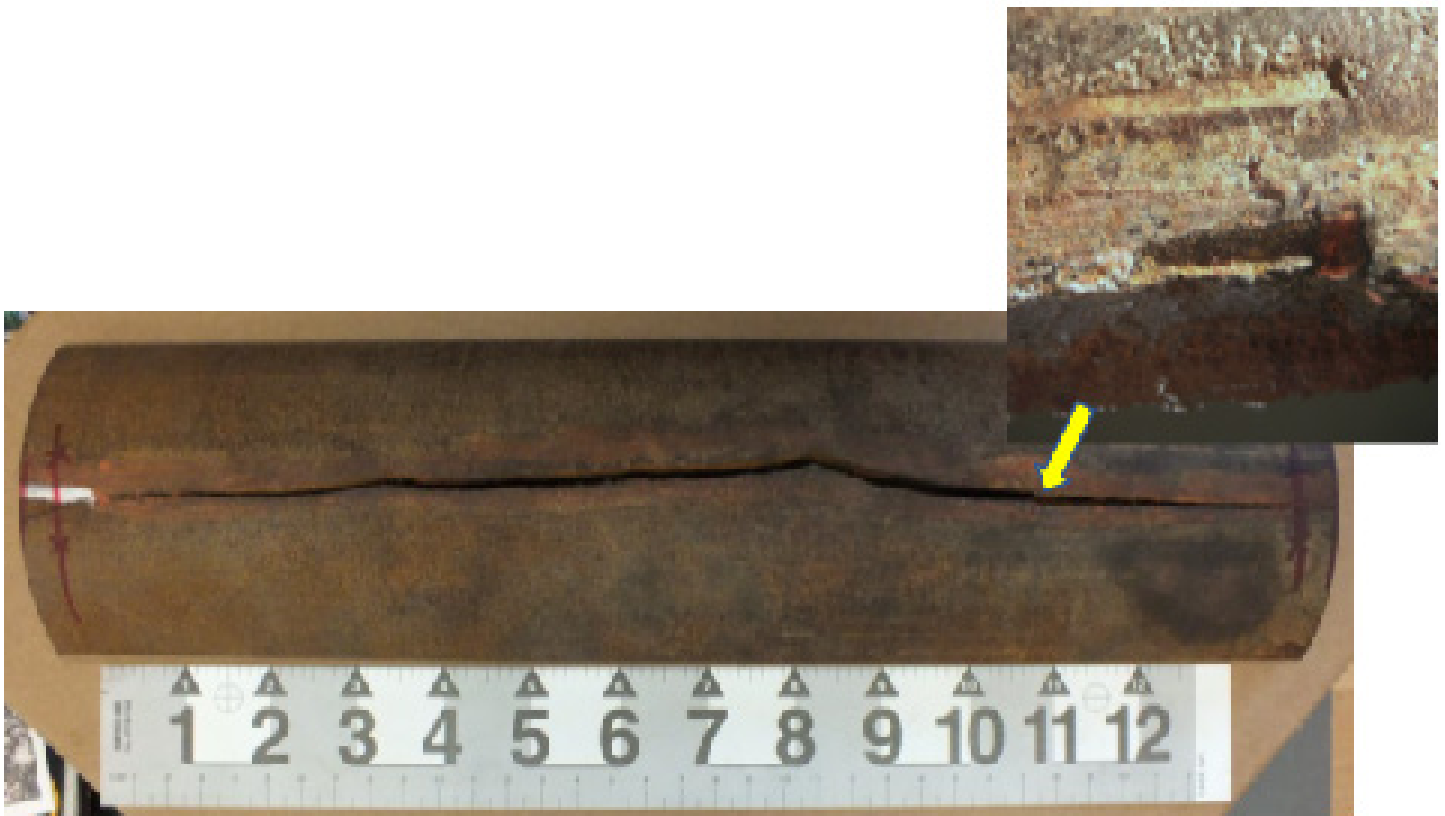
Figure: Photo of ruptured drill pipe (Insert: Magnified image of tool marks that initiated the rupture.) (RJLG image)
